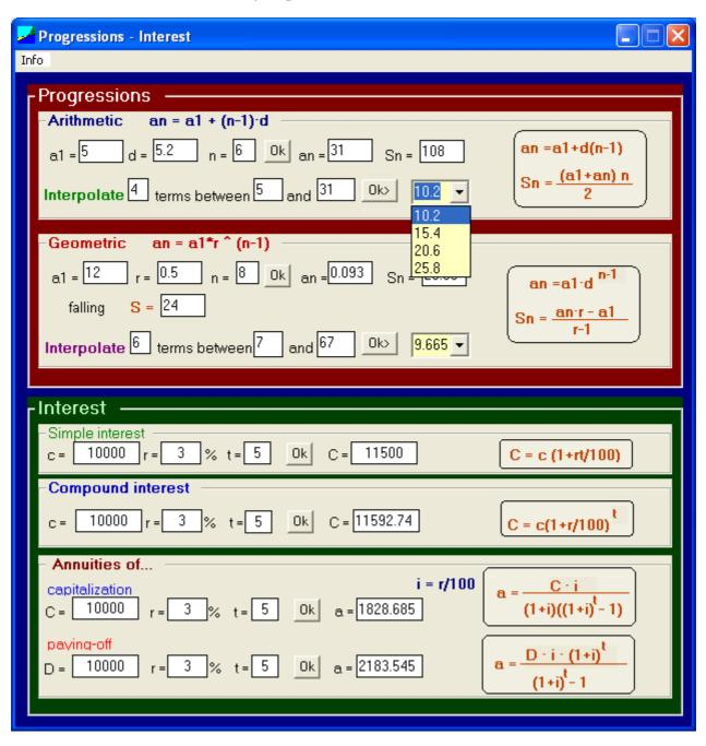
In all the cases it is necessary to introduce <u>3 data</u> and after pressing **Ok** the rest of parameters will be calculated.
